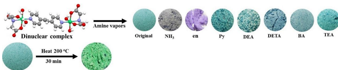
Figure 1. Crystal structure of the metal complex, the color changed after heating and exposure in various amine vapors.
