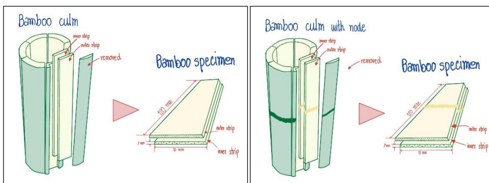
Figure 1 Specimen preparation for flexural test
