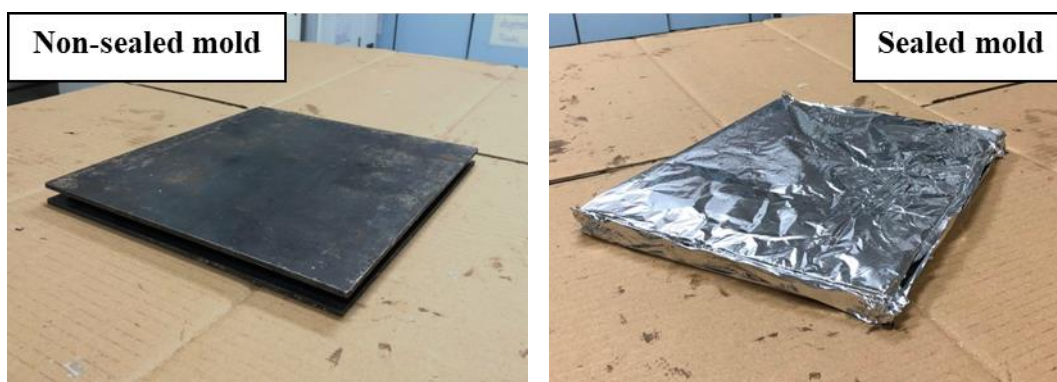
Figure 1. Photos of the non-sealed (left) and sealed molds (right).
