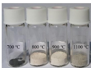
Figure 1. Photograph of obtained powders sample calcined at 700, 800, 900 and 1,100 °C
