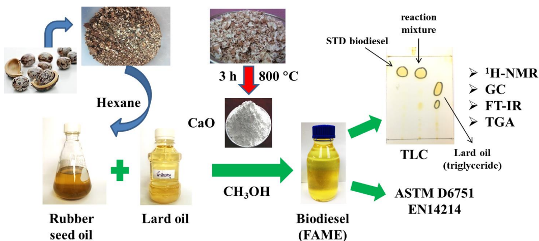
Figure 1. Rubber seed oil mixed with lard oil can be utilized as a potential feedstock in the biodiesel production process for using with agricultural diesel engines of Thailand.
