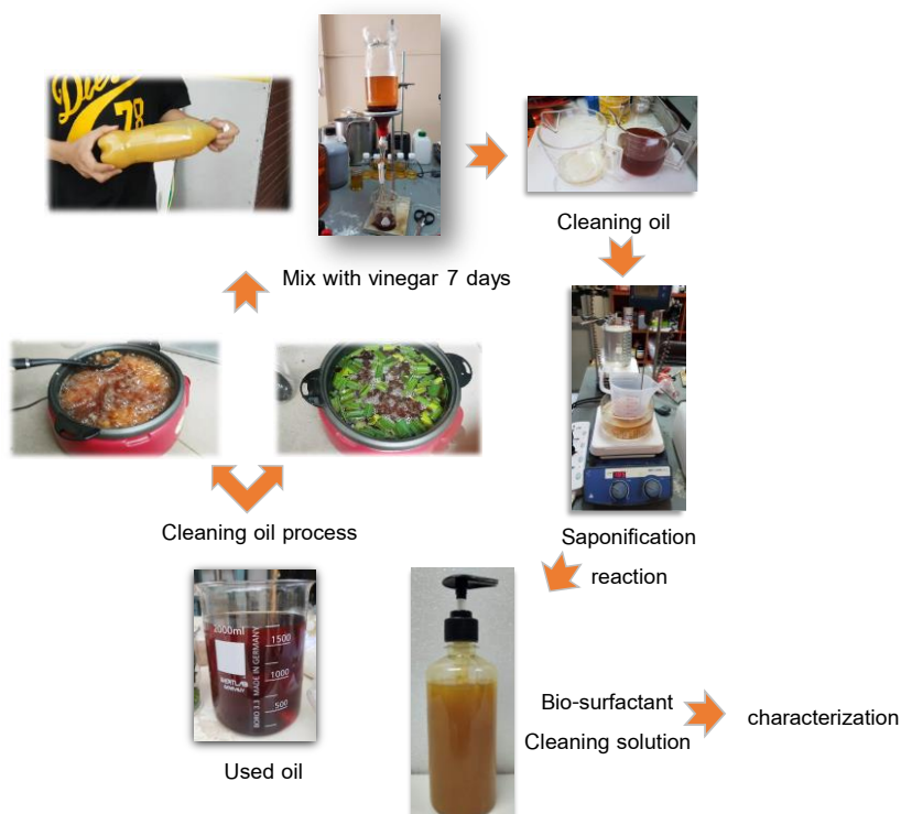
Figure 1. Graphical abstract shows the process of the producing of green bio-surfactant from used oil.
